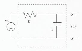
Analyze the circuit for  $t > 0^-$  given that the initial voltage across the capacitor is 0 V.
