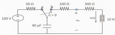
Determine  $v_0(t)$  by taking the Laplace transform of the circuit, and then solving for the time-domain expression.
